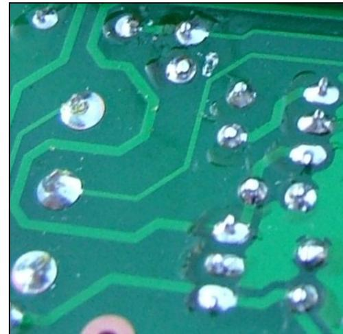
Where possible fit the components so their values are easily readable. Some components **MUST** be fitted in the correct orientation as they are polarised; this will be indicated in the text. The components are packed in
